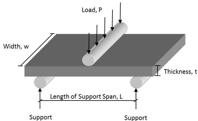
**Figure 1. Test set-up for a 3-point bending test**
