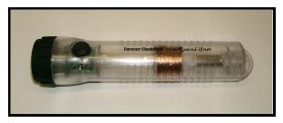
The Faraday Flashlight is a mechanically powered flashlight. The flashlight contains a powerful neodymium magnet that moves back and forth between a coil of copper wire. Energy is generated and stored in a supercapacitor. Shaking the flashlight back and forth for 30 seconds will provide about 5 minutes of light. (image)
